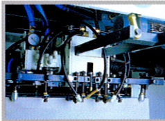
FEEDER With Suction Device in mechanical driving, sheets smoothly fed.
