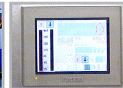
TOUCH SCREEN Clear and simple readings ensures quick fault finding and machine operation. Cutting pressure gauge ensures machine and cutting die durability by checking cutting pressure and over-cutting pressure.
