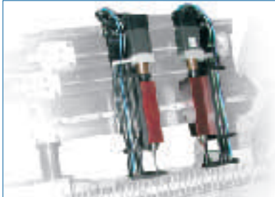
Dürselen PB.15 DoD: Automated drilling on demand
