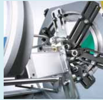
Fitted counter-pressure unit
