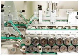
The modular side register system squares cartons prior to entering the prefold section, giving additional control over blanks. A driven upper and lower auxiliary carrier transports blanks through the section when the side register is not being utilized
