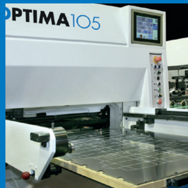
Fast Lock Die Chases and adjustable Counter-plate. Machine control by Touch Screen
