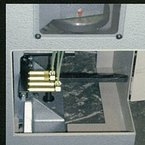
★ CENTRAL GREASE SYSTEM
