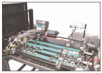
Vacuum Feeder Segmented Table Increases versatility for folding, gluing and converting jobs. The table design utilizes 2 inch wide segments joined together along the entire table length. These can be removed or replaced as required, to accommodate a wide range of jobs.
