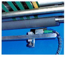
FOLD LENGTH MONITORS beneath the exit rollers on Stations I and II measure product coming out of the folding stations and stops the machine when the folded length is incorrect.
