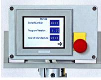
The touch-screen, color-graphical CONTROL PANEL (HMI) controls all the functions of the Vijuk outsert section—the knife folders, pressing unit, and vertical stacker—controlling speed, alignment, counts, and jam detection.
