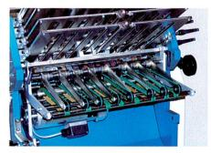
The independently controlled VARIABLE-SPEED TRANSFER UNIT carries the paper from Station I to Station II.
