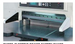
**PHOTO-ELECTRIC BEAMS SAFETY GUARD**A set of infra-red light beams is projected in front of the cutting zone just above the table to avoid accident.
