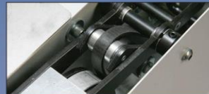
Simple positive tape drive, no eccentrics
