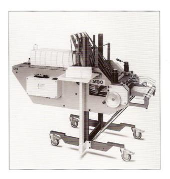
Vertical stacker delivery with pressing for one-up production. Integrated pressing with pre- and main pressing rollers. Solid and space saving construction, large loading capacity. Convenient sheet removing. The sheets are stacked upwards with their spine, therefore collating mark always visible to operator. Integrated batch counter for counting and marking.
