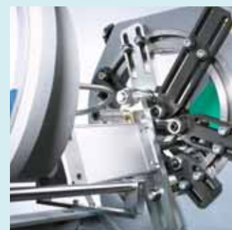
Fitted counter-pressure unit
