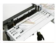
Automatic binding table clamps the media and holds the blocks in place during binding. It then ejects the book or calendar blocks automatically up to 60% more productive than a stand binding table.
