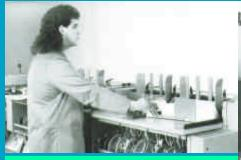
The feeder has both mechanical and vacuum opening. It handles a wide variety of sheet-fed or web signatures from 4 to 64 pages, cards, envelopes, with or without lap (lap pre-
