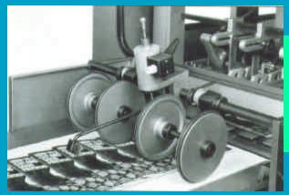
A counter and kicker on the belt delivery provide a gap in the shingle, making it easy to stack off batches of preset count. The number of copies in each batch is set on a preselector switch. A totalizer gives an accurate count of copies produced.
