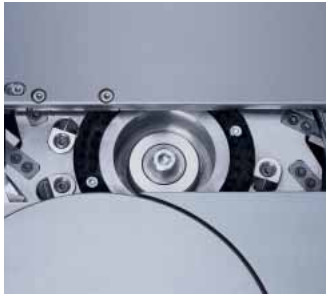
The combination tool of the spine preparation station of the Eurobind 600/600 PUR optimally prepares the sheet edges for gluing.
