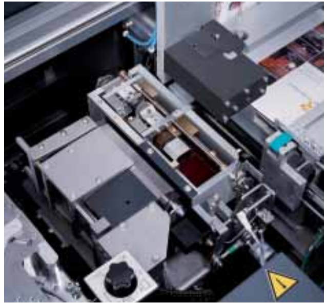
The glue nozzle technology of the Eurobind 600 PUR allows precise application of PUR adhesives.
