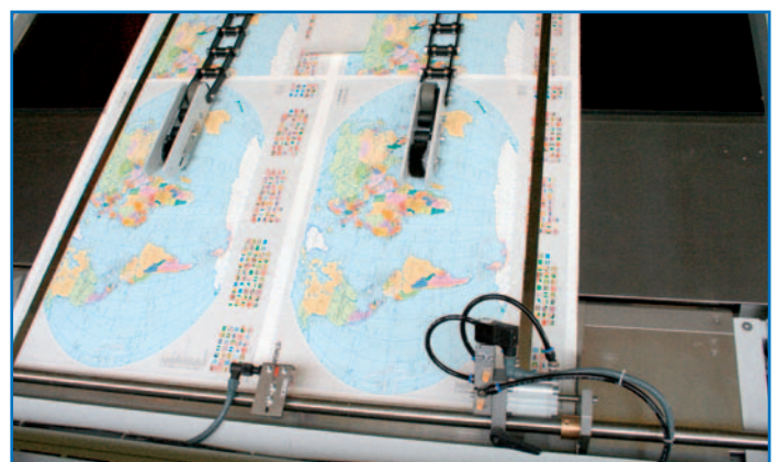
suction-belt feeder for substrate sheets
