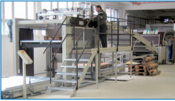
automatic laminator with down-stacker and pallet logistic
