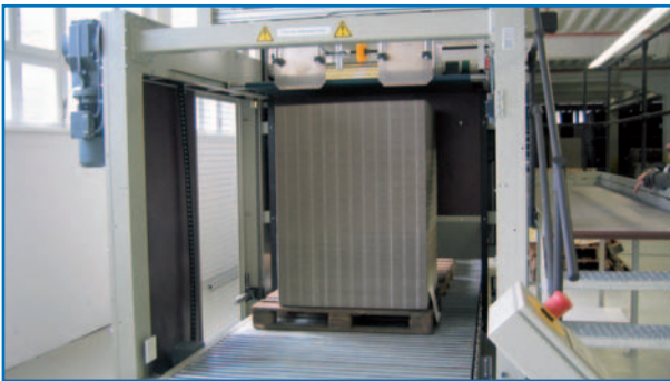
non-stop down-stacker with pallet logistics
