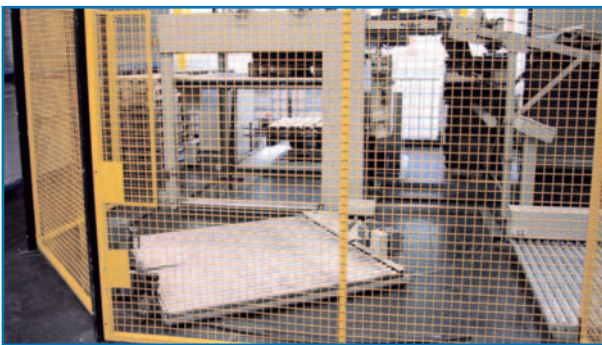
non-stop down-stacker with pallet logistics
