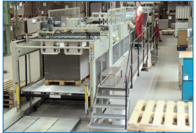
automatic non-stop down-stacker and flip-flop
