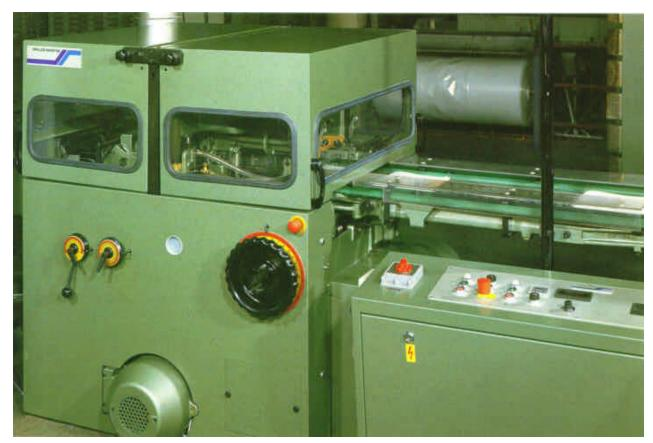
The 3-knife trimmer is an important component of an efficient production line. Saddle stitcher and 3-knife trimmer should be carefully matched to assure consistent output and product quality.
