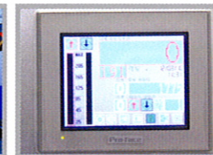
TOUCH SCREEN Clear and simple readings ensures quick fault finding and machine operation. Cutting pressure gauge ensures machine and cutting die durability by checking cutting pressure and over-cutting pressure.
