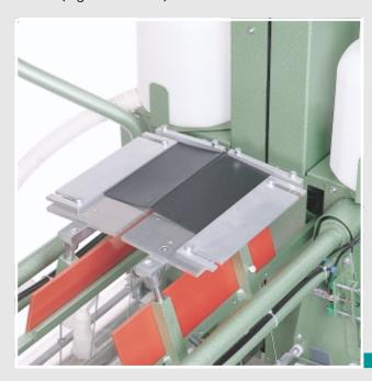
The second is a table-top unit that is used instead of the normal case-guide for small, soft and hardback book covers. This unit in the form of two side table-top boards is far more intricate, but is therefore more suitable for soft cases. The cases are flatly positioned, here
