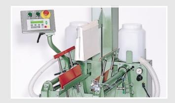
The casing-in cycle is next triggered. A push button in the control panel serves to this end. The blade drives downwards between the glueing units.
