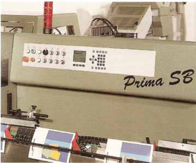
Prima SB operator control with full PLC interface with display, fault readout, speed readout, and make-ready assist.
