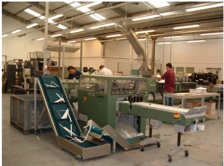
Conveyor system KF 145 with HF 35 on Müller Martini Minuteman
