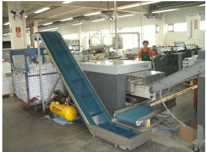
Waste conveyor KF 175 with HF 00 on Heidelberg Stitchmaster
