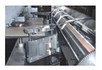
The Corner Trimmer Option automatically trims the Corners from the cover material very accurately during the casemaking operation. This feature streamlines production for On-Demand and Ultra Short Run applications while providing high quality, uniform corners on every cover—even in runs of one!
