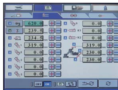
The guide and buckle positions can be fine-tuned by 0.1 mm using the + or - button.
