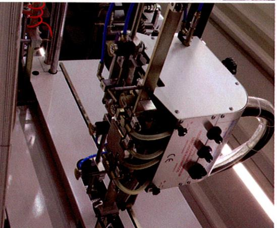
*Elimination of electrostatic charges through blowers with ionised air, electrostatic bar and autonomous power supply unit. Pneumatic or pinch-pull square with vacuum force regulation vacuum force regulation for a perfect alignment of the sheets on the register gate.*
