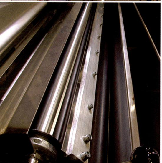
*Pneumatic expandable film rolls shaft, swivable for easy exchange of film roll.
