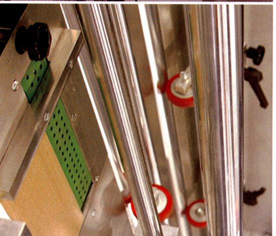
*Cutting system with the hot rotating blade, for in-line separation at high speeds of films in polyester, nylon, embossed, holographic and metalized.*
