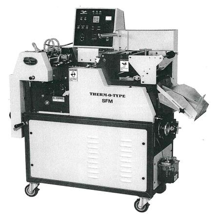
The SFM has become a proven performer in the foil stamping industry. Proven in some of the highest production plants in the country, the SFM offers exceptional productivity, fast set-up and ease of operation.
