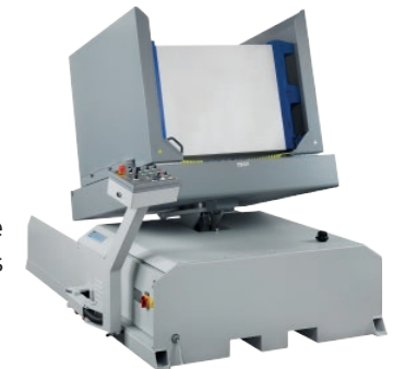
Rear side removal of bad sheets
