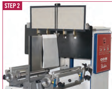
Open cover is inserted into the cover guide. The spine portion of the cover is held in place with vacuum. Book block is placed on the wing.
