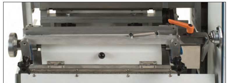
Optional: Extra paste attachment deposits additional adhesive in joint area.
