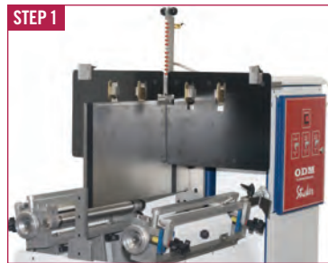
Casing-in thin books on a blade based casing-in machine has always been a difficult and tedious task. Now with the cover guide, the accurate placement of thin covers is a snap. In addition, it saves production time, eliminating the manual operation of 'pre forming' the covers.
