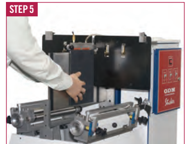
After the book is closed, the vacuum arm is (manually) returned to the home position and the book is removed from the wing.
