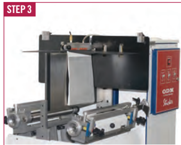
When the wing returns back to the home position, the cover guide bar is (manually) lowered to contact the spine of the book block.
