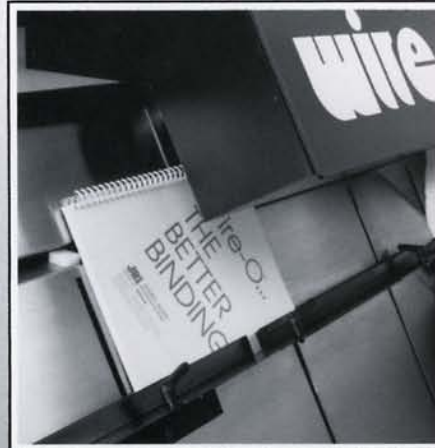
Wire-O Binding is closed automatically
