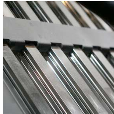
The new Stahlfolder buckle with solid paper stop is designed to increase speed and fold quality
