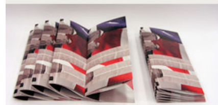
Pressing deliveries provide a better product for further bindery processing, i.e. for stitching or perfect binding
