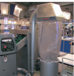
TRIM WASTE SYSTEM
