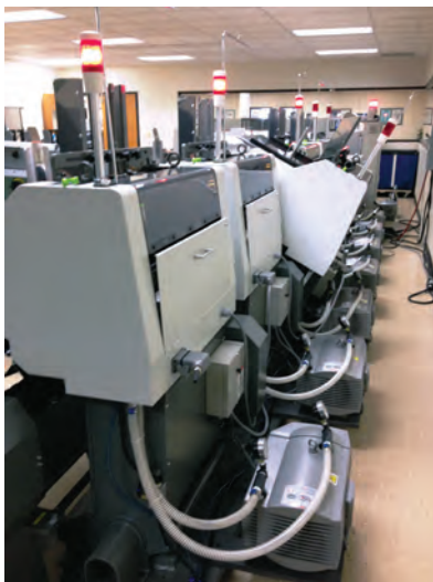
Rotary feeders – tilt back/tilt forward feature with individual pumps
