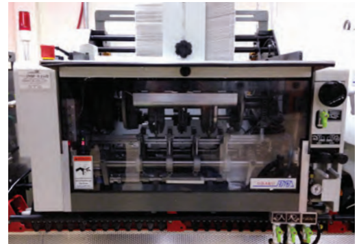
Rotary feeders – toolless setup, backstop and vacuum timing adjustable on-the-fly
