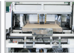
FEEDING SECTION Precise feeding of product by suction device. Automatic setting of side joggers on Touch Screen.
