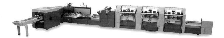
the pile and marking is largely avoided. The signature is fed neatly and reliable at the register, no setting operations are required. Signatures can be fed three ways; Vacuum Opening-Signatures with closed head or tail are reliably opened by suckers, High Folio Opening-Signatures with high folio lip (min. 1/4"/6 mm) are processed, Low Folio Opening-Signatures with low folio lip (min. 5/16"/8 mm) are processed.
