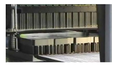
2. A series of approximately 5,000 upper and lower pins facilitate the separation of finished cartons from waste scrap, with upper pins pushing the waste down while lower pins secure the finished product.
