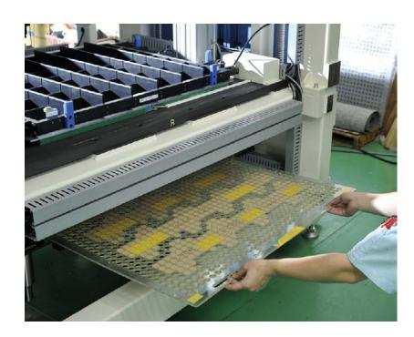
1. A stack of 2.5 - 3" of die cut sheets register to the infeed guide
