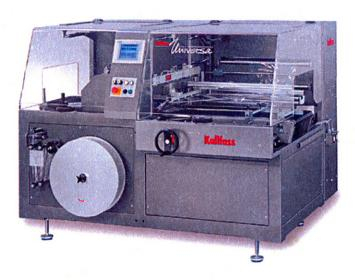
Innovative technology makes the **UNIVERSA 400** fast and versatile to deliver a smooth and precise packaging process with speeds up to 70 packs per minute.
