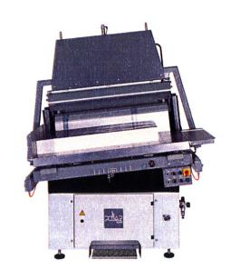
machine output is considerably increased. The precise alignment of the material to be cut, and the resulting improved cutting accuracy lays the foundations of a uniform and high quality of the final product. The air removal feature improves the formation of blocks from the reams to be cut and reduces the production risks once more. With the automatic jogger positioned directly next to the rear table, unloading can be performed automatically via a gripper system.
