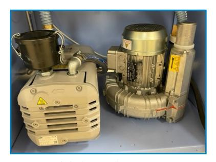
Separate high volume air and vacuum pump systems
