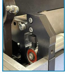
Steel side frame construction for superior strength, minimal maintenance, and longer life.
