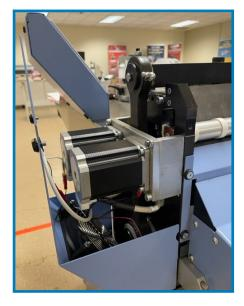
Quick and quality stepper motors are utilized, as apposed to belt and pulley systems, which are capable of achieving up to 14,000 sheets per hour.
