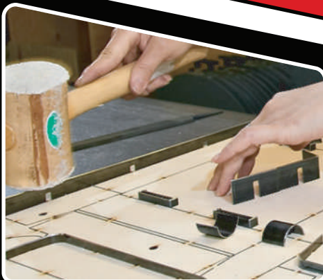
Upper: Steel Rule dies produced by pre-bent metal cutting blades being inserted into notches cut into a wooden base.
