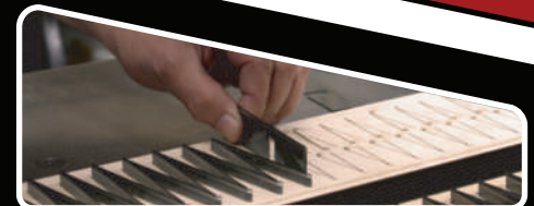
Upper: Steel Rule dies produced by pre-bent metal cutting blades being inserted into notches cut into a wooden base.
