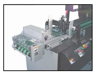
Convert the KR 215 into an inline transport using the KR 412 Shuttle By-Pass and use it inline with folders, tabbers, etc.
