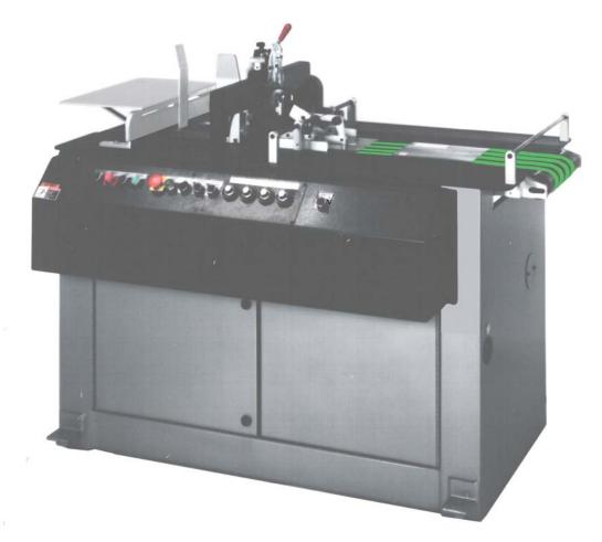
Feed and convey a wide variety of products using the KR 215 IJ. Used with most major brands of inkjet printing and pressure-sensitive labeling equipment, the KR 215 is the ideal feed and transport solution for your offline coding, addressing and labeling needs.
