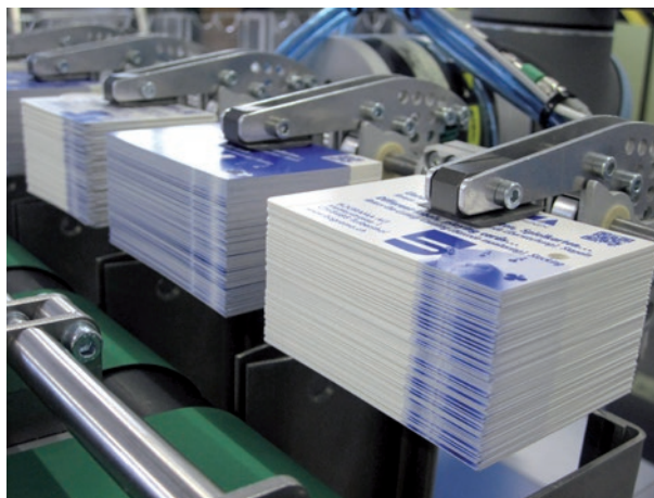
BSR 550 Servo in combination with „RoboStack“; Automated sorting and packaging solution for filling trays, banding or placing on a belt.
