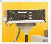
The Registron S 3920 PCR « Kurandt » glue-line detector ensures perfect monitoring of the presence and quantity of glue on the lower line.
