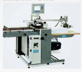
• **P4 or P5 Pallet Feeder** A pallet stacked with up to 47<sup>1</sup>/4" of paper can be loaded directly onto the feeder, saving time and labor. A laser beam automatically positions the pallet for transferring sheets onto the stainless-steel alignment table by rear suction pickup and a drum suction wheel. Setup and operation is through L4 and M4 Controllers.
