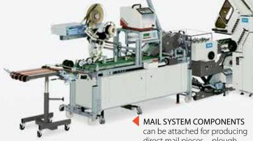
can be attached for producing direct mail pieces—plough folders, card feeders, labeling, wafer sealing, ink jetting, tipping, optical recognition, die punching, cutting, glue systems, and vacuum belt transports.
