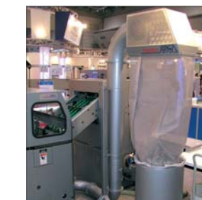
TRIM WASTE SYSTEM
